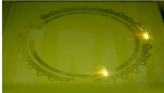
Picture 1.1: Laser sintering a component with internal design features
