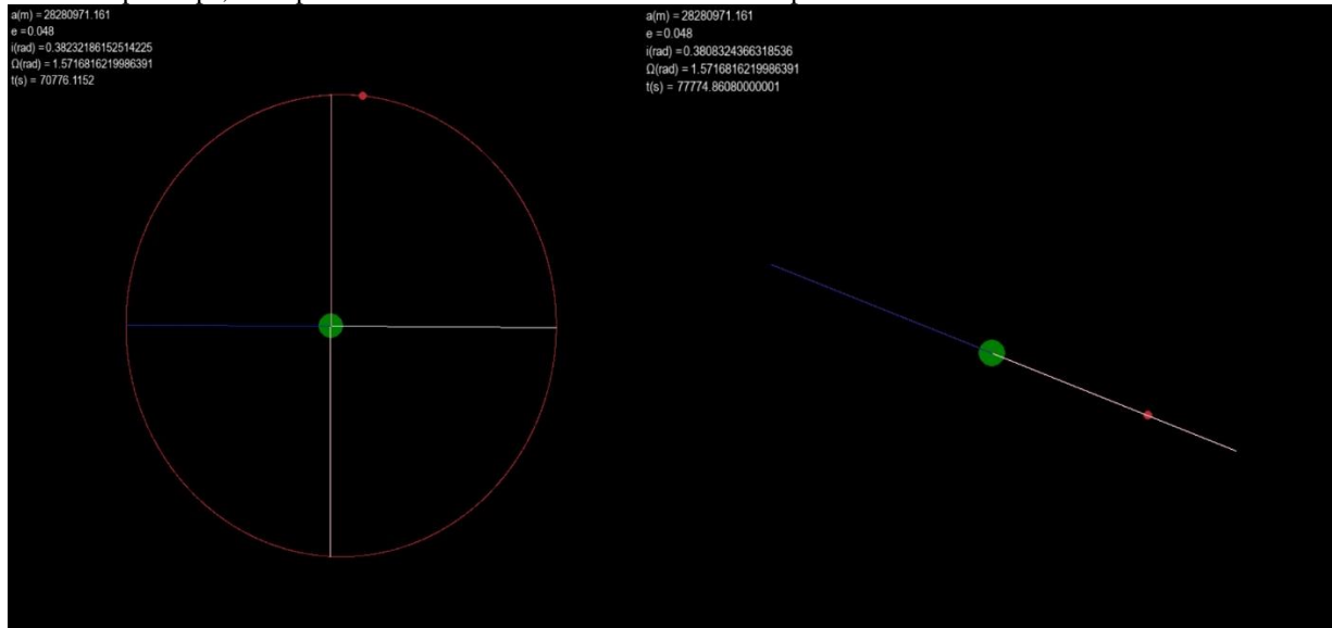
Fig. 6. The illustration of a debris' orbit returned by the simulation. The image on the left represents the trajectory as seen from the top of the Moon's orbital plane and the image on the right is the orbit viewed from an observer inside the Moon's orbital plane. The top-left corner of each image contains important orbital parameters, such as the pseudo- semi-major axis and eccentricity, the longitude of the ascending node and the elapsed time.
