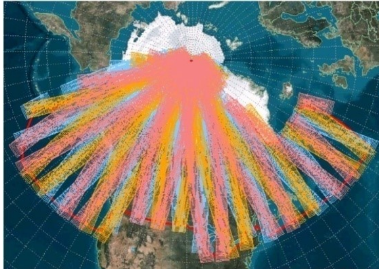
Figure 1. Twenty-four hour coverage of Canada and northern polar regions; RCM satellites 1, 2 and 3 in blue, pink and orange respectively
