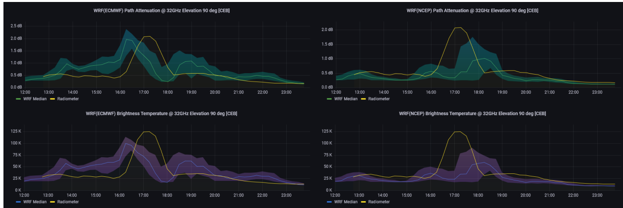
Fig. 4 Grafana: example of comparison of forecast (in green and violet) and measured (yellow) radio-propagation products, Cebreros, November 2022.
