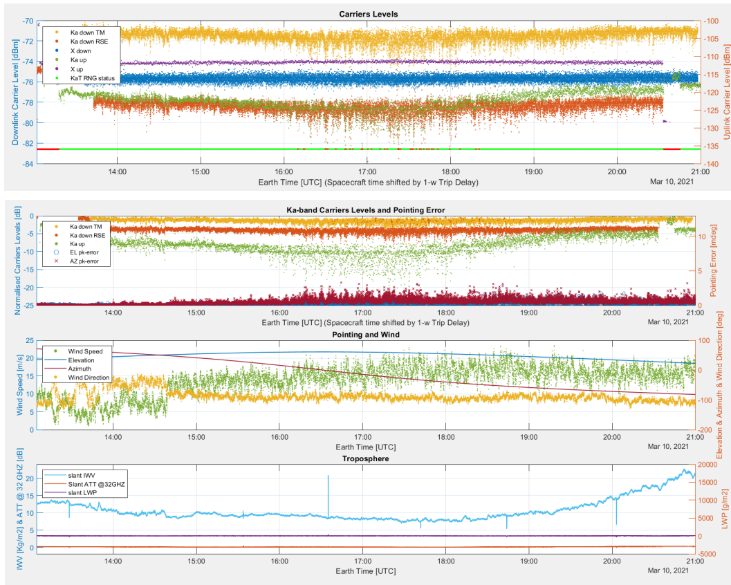
Fig. 3. Ground and Spacecraft data from first day of SCE#1 (pass on DOY 069)
