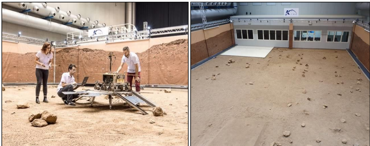
Figure 15 – The Mars Terrain Simulator (MTS); ExoTeR Rover – ESA property
