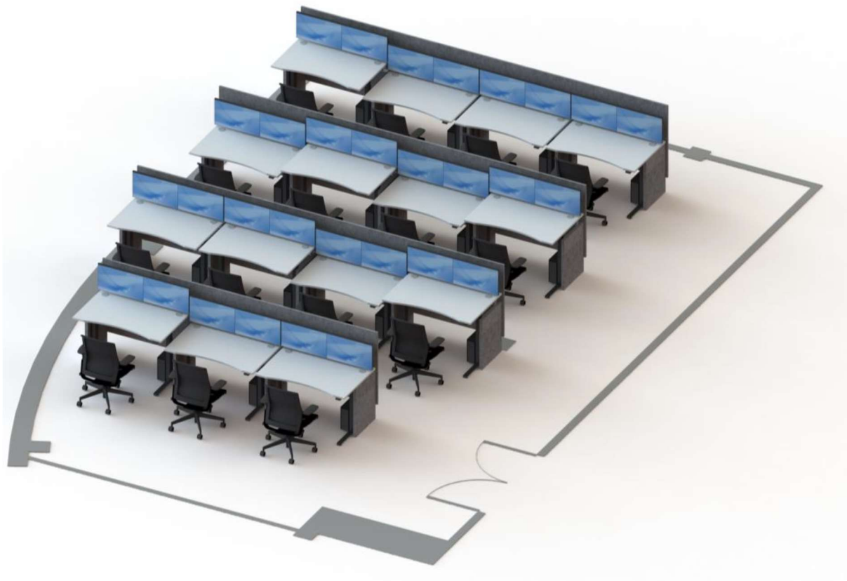
Figure 4 Working Consoles in Main Control room
