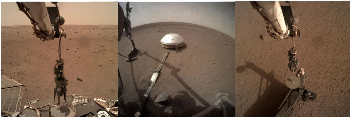
Figure 4: HP 3 deployment onto the martian surface by the robotic arm of the lander. Left: Sol 74 – HP 3 capture by the robotic arm; middle: sol 76 – HP 3 placement on the surface; sol 83 – Grapple release of HP 3 [credit NASA/JPL-Caltech]
