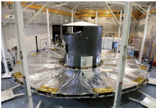
Fig. 1. Gaia Deployable Sunshield Assembly fully deployed at Astrium Toulouse (Copyright Astrium)
