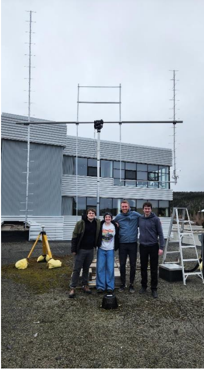
Figure 10: Assembled M2 Yagi Antennas on the roof of C-Core Office in St. John's, NL [7]
