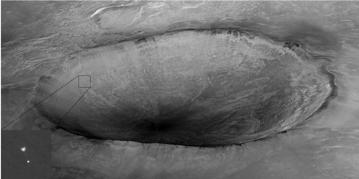
Figure 14: MRO’s HiRISE camera was able to capture the Phoenix lander on its parachute during its descent, a feat that was the result of both good engineering and good luck. The pointing of MRO was optimized to acquire the radio signal transmitted from Phoenix assuming a wide variety of possible landing trajectories, and the time when the image was taken was estimated based on these trajectories in an attempt to capture the lander as it passed through the imager’s field of view. It worked! It is noted that Phoenix did not land in the crater in this image (Heimdall crater), but instead in Vastitas Borealis. This was the first time a vehicle’s descent onto a non-terrestrial body was captured in an image. Credit: NASA/JPL.
