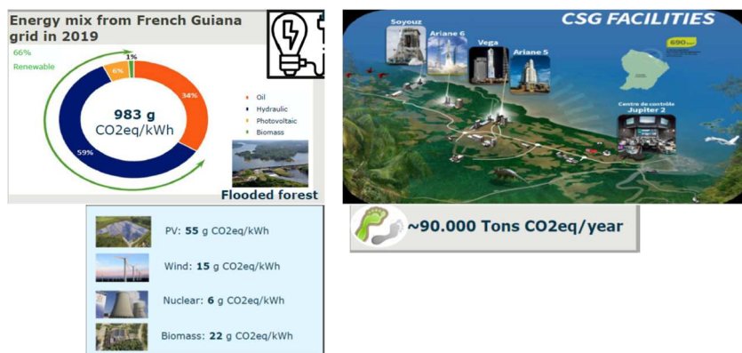
Figure 4 : Carbon footprint emissions from power grid consumption
