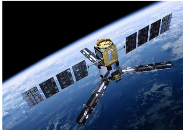
Fig. 1. Artist's impression of the SMOS flight configuration, illustrating both the Microwave Imaging Radiometer using Aperture Synthesis (MIRAS) payload and the Plateforme Reconfigurable pour l'Observation, les Télécommunications Et les Usages Scientifiques (PROTEUS) platform. (source: AOES Medialab, ESA)
