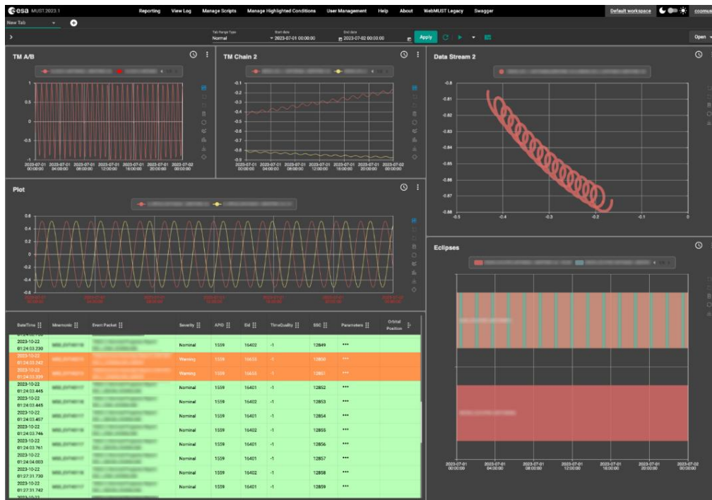
Figure 1. Screenshot of NGWebMUST displaying a dashboard combining housekeeping telemetry displayed as single linear plots, textual data as Bar Charts, a XY Correlation plot and a table containing the history of events registered on-board.
