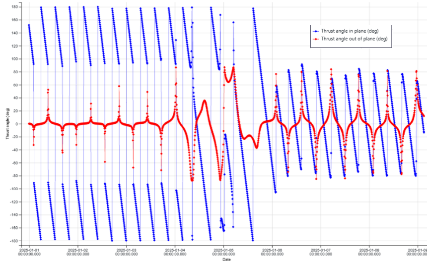
Fig. 7: Thrust in and out of plane angles for relocation with Sun illumination imposition
