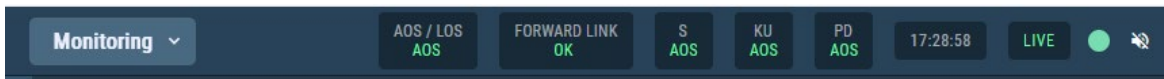
Figure 3 AOS/LOS indicators as well as TM reception indicators have been added to increase operational awareness of the current connection status between the ground and space segment
