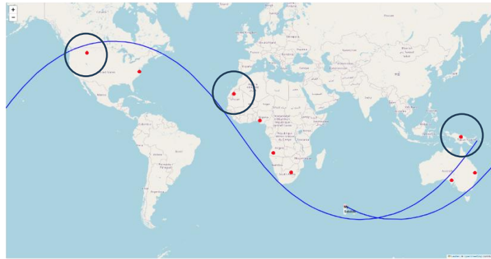
Fig. 2. Satellite Ground Track with Client Ground Station Locations
