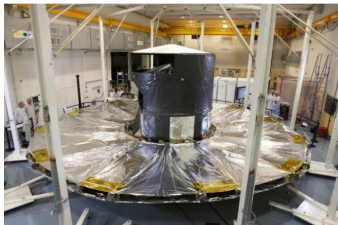
Fig. 4. Gaia in the fairing (left), and with the Deployable Sunshield Assembly (DSA) fully deployed at Astrium Toulouse (right)
