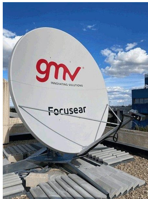
Figure 4: GMV’s Focusear passive ranging antenna in Madrid
