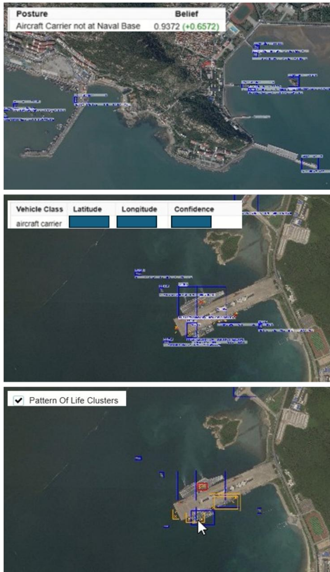
Figure 6: CASTT Demonstration Mission. From top to bottom: 1) Initial collect reveals no ship where one was previously expected, 2) Follow-up collection on a different port detects the ship and 3) Ship detections from follow-up collection are compared with POL for that port determined from historical data on that location.
