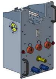
Fig. 6. 3D modelling of MiF insert
