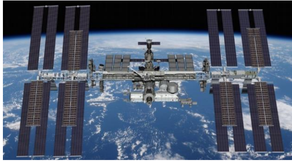
Fig. 10. ISS total solar power system as of June 2023, composed of the 16 original solar panels and 6 new iROSA panels. (Credit: NASA)
