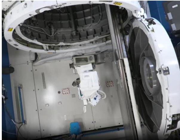
Fig. 4. CLPA camera waiting on the JEM slide table to be retrieved by Dextre. (Credit: CSA)
