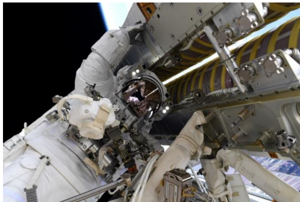
Fig. 8. Astronaut Shane Kimbrough holding iROSA panels during first deployment. (Credit: NASA)
