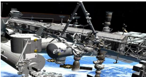
Fig. 6. Visualisation of Canadarm2 and Dextre and their limited clearance to other ISS modules during three-way camera swap. Image acquired during simulation with CSA 3D-visual model MOTS (Credit: CSA).
