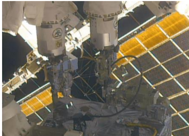
Fig. 3. Dual-arm operation by Dextre during RRM3. (Credit: NASA)
