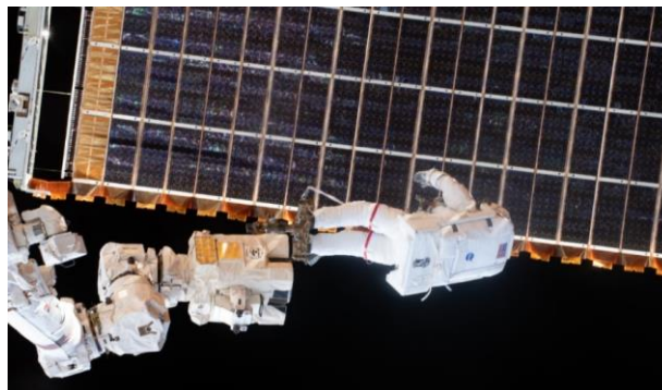
Fig. 9. Astronaut Thomas Pesquet into an APFR performing precise technical tasks for the deployment of solar arrays.
