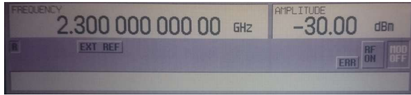
Figure 4.2: Signal generator set within the band of interest.
