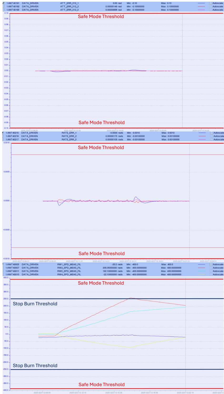
Fig. 5. Attitude Error, Attitude Rate Error and RW Speed for Safe Mode case
