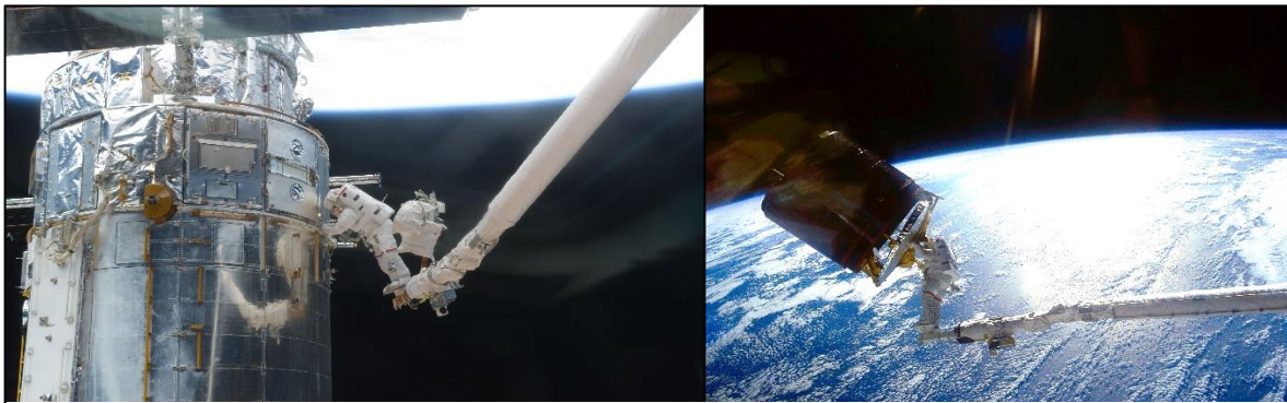
Figure 2 - SRMS Use for EVA Satellite Repair and Capture. Photos courtesy NASA.
