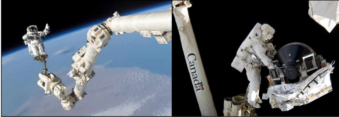
Figure 3 – SSRMS-supported EVA. Photos courtesy NASA.
