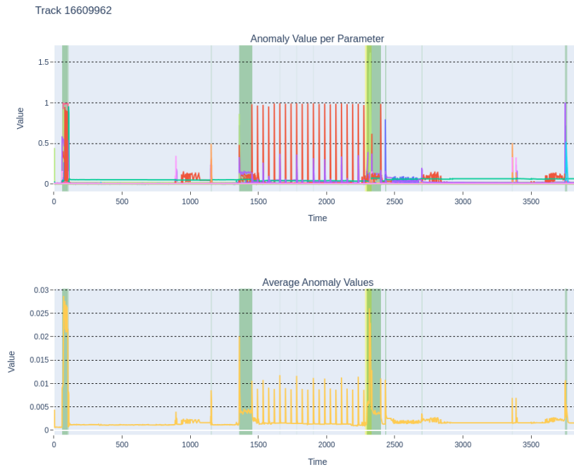
Figure 2: Example of TranAD+ labeling anomalous regions (green) on an anomaly labeled (yellow) track from DSN 1k.
