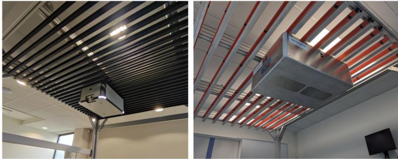
Figure 5: Small-size CeiliX vehicle, battery powered (left), and Medium-size CeiliX vehicle, ceiling powered (right)
