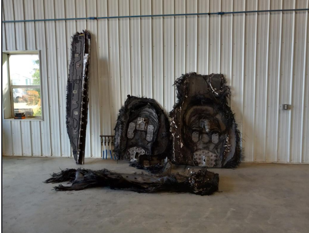
Fig.13. Fragments from the trunk recovered near Ituna and later returned to SpaceX. The tallest object on the left is approximately 2.5 meters in length. Image credit Dr Sam Lawler [13].
