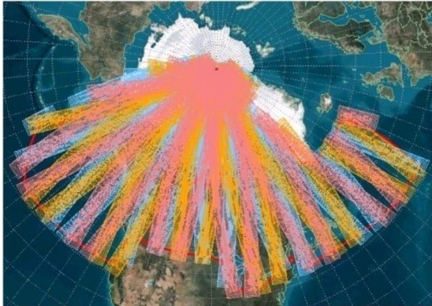
Fig. 1. Twenty-four hour coverage, Canada and Northern polar regions, RCM satellites 1, 2 and 3 in blue, pink and orange respectively.
