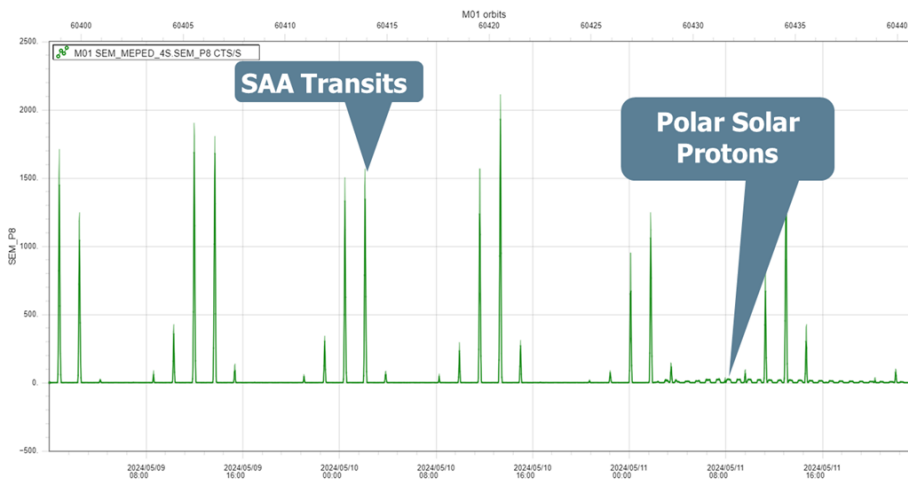
Figure 11. 70MeV proton flux measurements from the SEM-2 instrument onboard MetOp satellites during the geomagnetic storm on May 11, 2024. The plot distinguishes between increased proton fluxes associated with polar solar storm activity and those detected during South Atlantic Anomaly (SAA) transits. The SAA-related fluxes exhibit significantly higher intensities compared to those originating from solar events.
