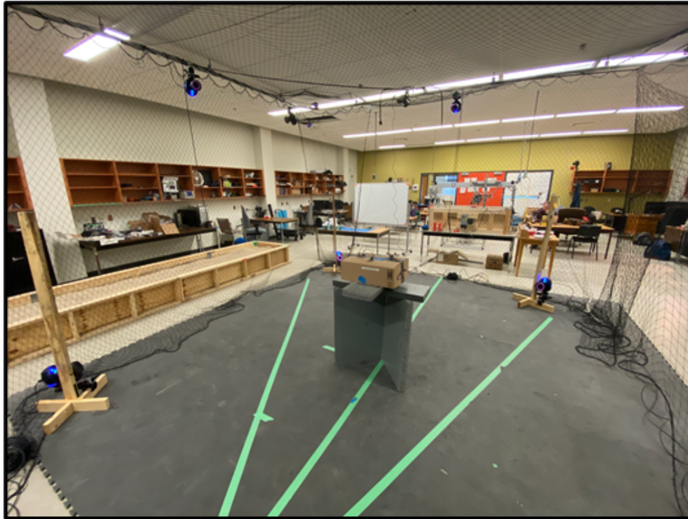
Figure 2: Overview of the VICON motion capture laboratory. The netted capture area is surrounded by 12 cameras arranged to track reflective markers at 100 Hz.
