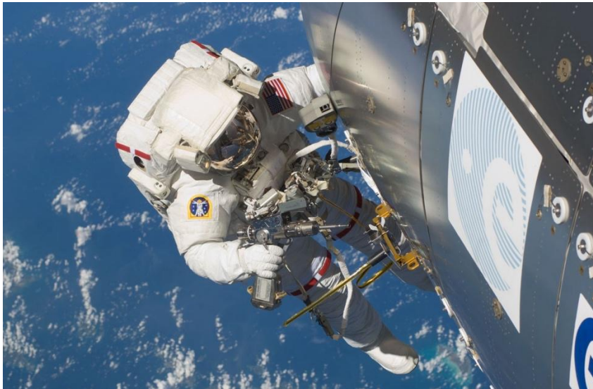
Fig 2. The Columbus Module VHF/UHF antenna being installed by Astronaut Randy Bresnik
