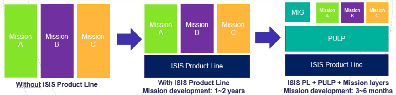
Fig 3. Stacking layers to reach a full operational control center
