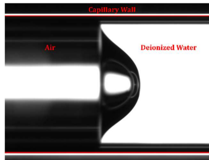
Fig. 2. Sample image of the air-water interface, with water volume of 0.1mL, and at 4500RPMs.
