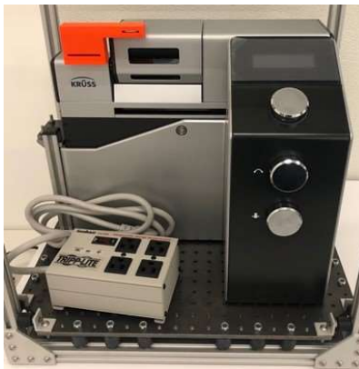
Fig. 1. KRUSS SDT, sitting in a vibrationally dampened frame designed for the parabolic flight.
